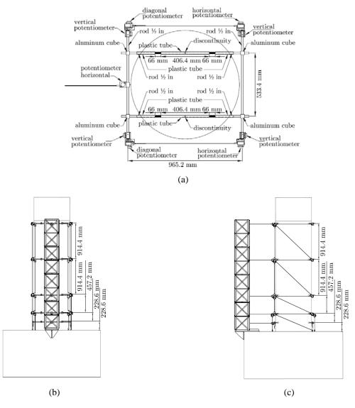
Figure 4: External instrumentation: (a) typical section plan view, (b) front elevation view, and (c) lateral elevation view
