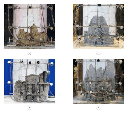
Figure 7: Damaged regions for all specimens: (a) CH300, (b) CS110, (c) CH300s, and (d) CH110.
