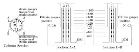
Figure 5: Internal instrumentation.
