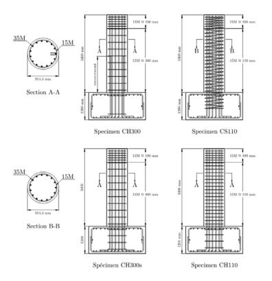
Figure 3: Specimen geometries. Table 1. Specimen properties
